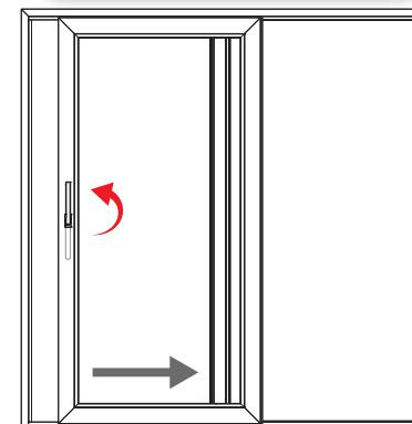
When the handle is lifted up, the sash moves away from the frame by 6 mm, after which it can be pushed to the side.
