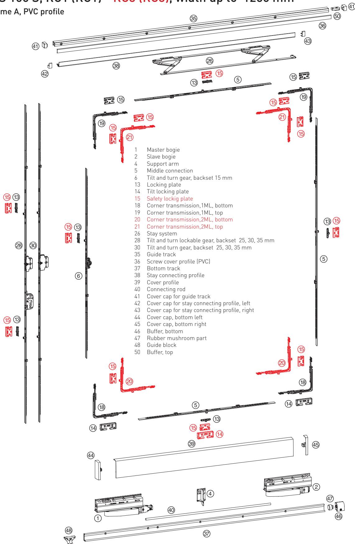
Figure fitting parts = design left (according to DIN EN 12519 opening to the right)
